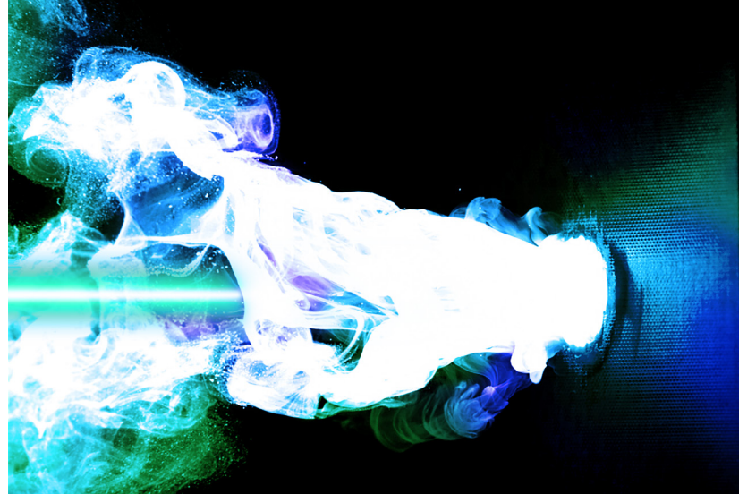
Formation of a vapor cloud in a laser-irradiated sample made of carbon-fiber-reinforced plastic. © Fraunhofer EMI
