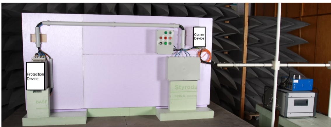
Figure 3: Horizontal orientation of the wiring loom – setup 2
