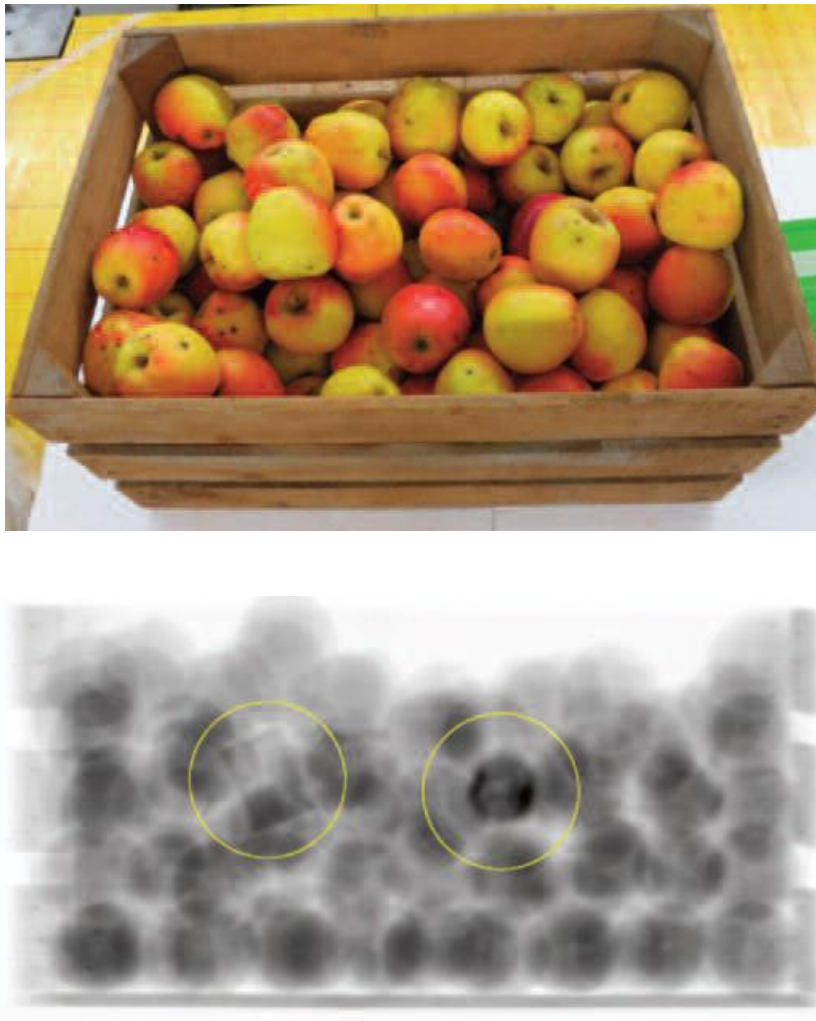
Figure 2: Example of images containing threats. Plastex and hand grenade hidden between apples. Photo (top) and X-ray image (bottom)
