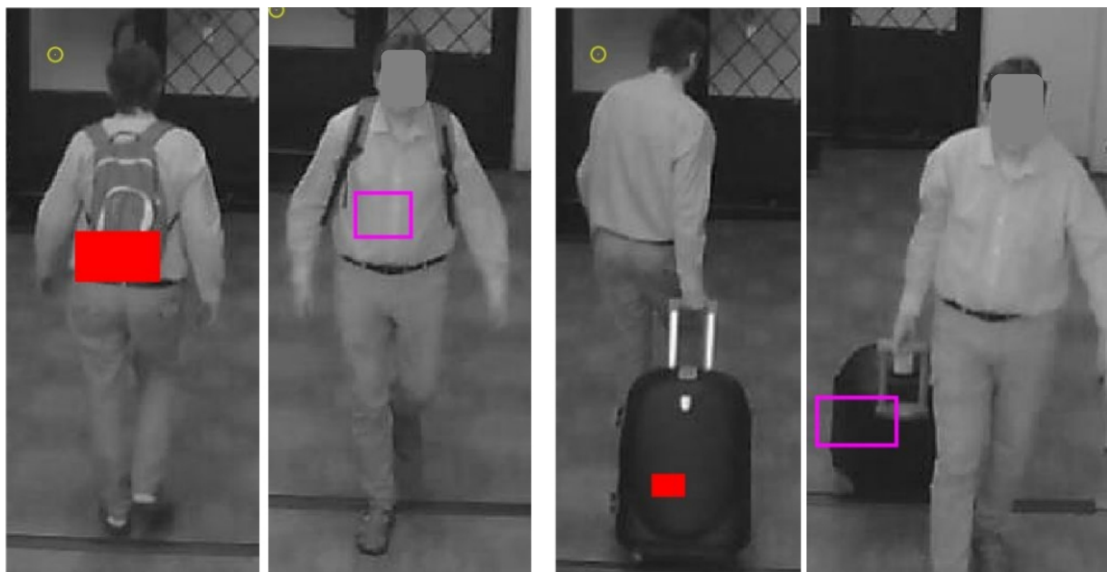
Figure 6. Examples of the images available to the user showing locations of threats in luggage. Filled red squares indicate that the threat is visible to the camera; open magenta squares indicate that the threat may be obstructed from the camera by the body.
