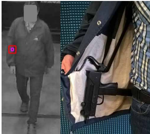
Figure 2: Detection of a concealed machine gun. Photograph shown on the left accompanies alarm information, which is sent to the remote user.
