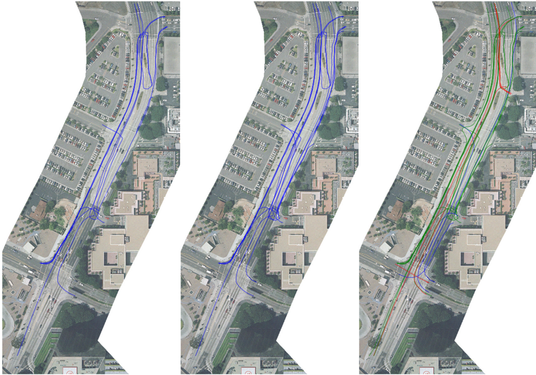
Fig. 3: The results of the anomaly detection in the Lankershim dataset. From left to right: LOF, FBOD and a comparison of the two algorithms. The blue trajectories in the left and middle figure are abnormal trajectories detected by the algorithm. In the right figure, green trajectories are the ones detected by both algorithms. Red trajectories are detected by LOF and blue ones are detected by FBOD.
