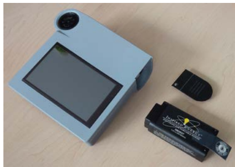
Fig 2: MobilePass Device with exchangeable battery
