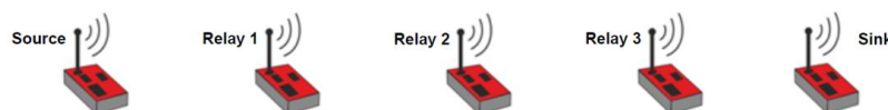
Fig. 3: Test setup consisting of source node, sink node and three relay nodes. Wake-up is only possible for neighbouring nodes, data transmission is possible directly from source to sink.
