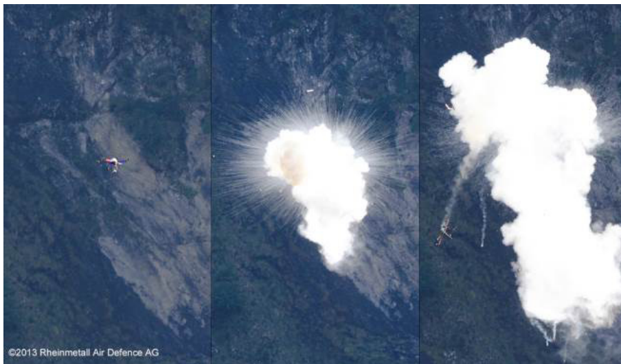
Fig. 4: Engaging a UAS with by the Mobile Effector Wheel XX. Frame series show the destruction of a VTUAS with an explosive payload.
