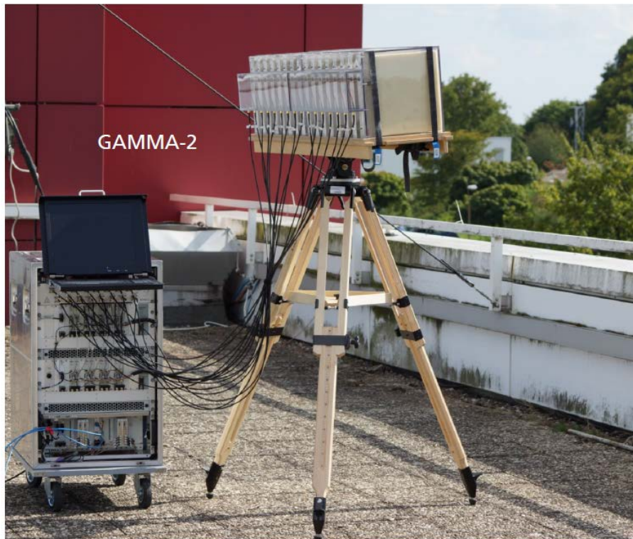
Fig. 4: Experimental passive radar exploiting six illuminating GSM base stations. In the measurement campaign, GPS-loggers provided the ground truth.
