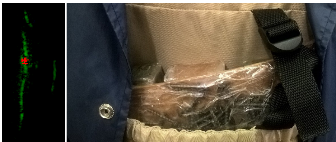
Figure 3. Detection of a “suicide belt” surrounded by shrapnel; a sequence of images similar to the one showed on the left are processed internally by the system to produce an alarm.
