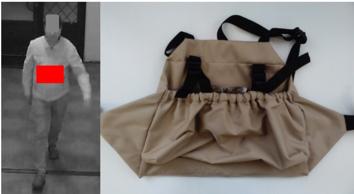
Figure 4. Example of detection of a mockup "suicide belt" with two small bricks of dielectric explosives' simulant. The location of the threat is shown by a rectangle superimposed on a photograph.
