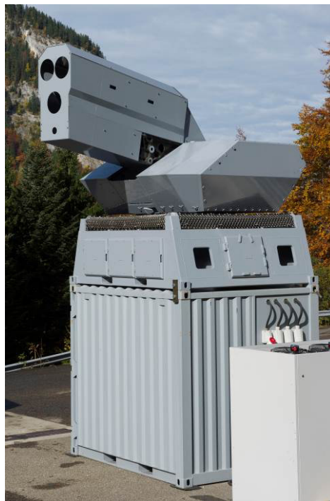
Fig. 3: Stationary demonstrator with 30 kW optical output power.
